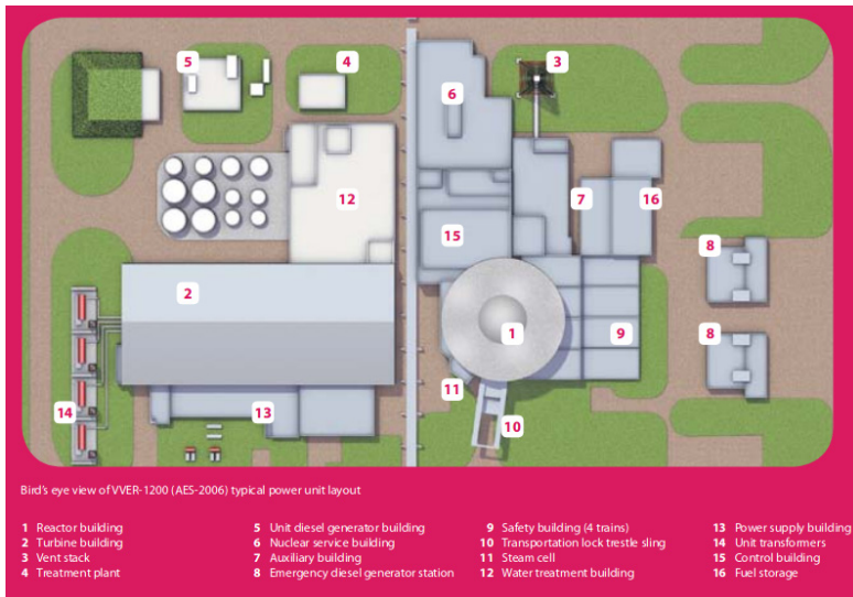
Fig (3): Bird's eye view of VVER-1200 (AES-2006) typical power unit layout [source: ROSATOM]
