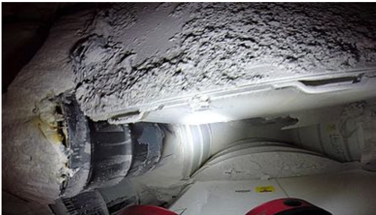
Fig (18): Damaged drum with radioactive waste inside WIPP, New Mexico, USA. The picture was taken on 2014-05-15 during investigations for the cause of radioactive contamination. Site is Panel 7, Room 7 [Source: Wikimedia]
